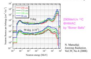
Distance dependence of neutron fluence for the incidence of C-290MeV/n in water.
